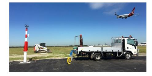
Working to a tight completion deadline, Pensar delivered a new runway visual range system that allowed for the safe landing and take-off of aircraft in low visibility at the Brisbane Airport.
